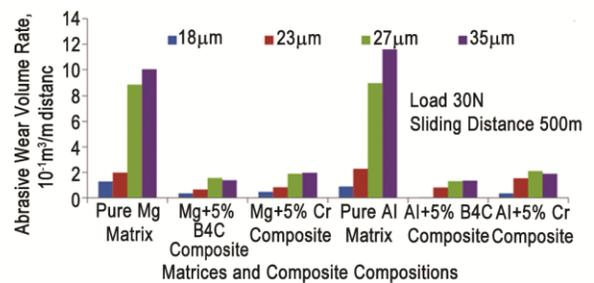
Fig. 4 — Wear rate of fabricated composites for 30N Load at 500 m
