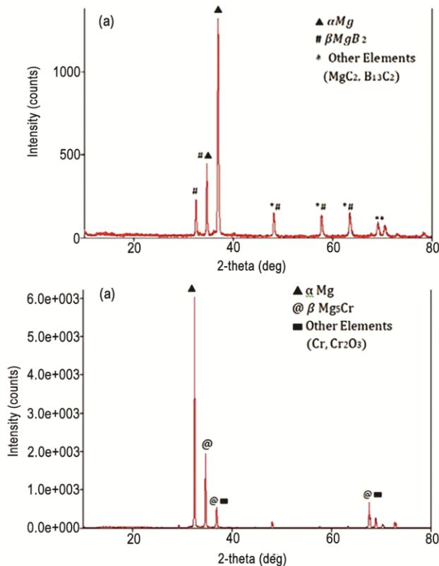
Fig. 2 — Diffraction images of (a) Mg-5%B<sub>4</sub>C composite, and (b) Mg-5%Cr composite
