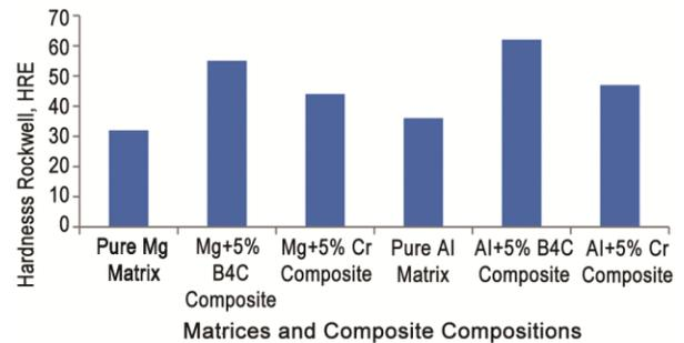
Fig. 3 — Hardness of Mg- and Al-matrices based composites
