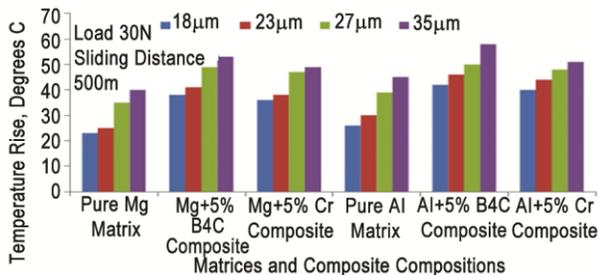
Fig. 5 — Abrasion Heating of Fabricated Composites for 30N Load at 500 m
