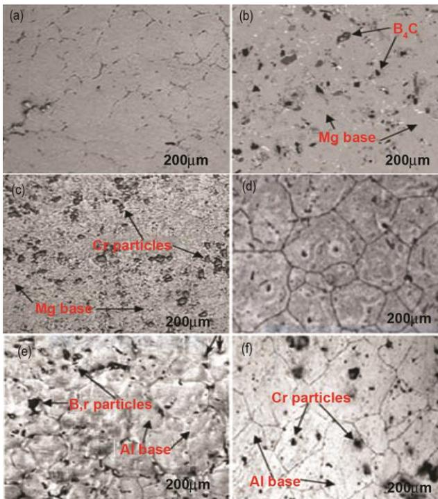
Fig. 1 — Microstructural images of (a) Mg-matrix, (b) Mg-5%B<sub>4</sub>C composite, (c) Mg-5%Cr composite, (d) Al-matrix, (e) Al-5%B<sub>4</sub>C composite, (f) Al-5%Cr composite
