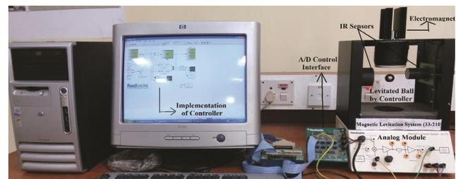
Fig. 1 — Maglev laboratory setup
