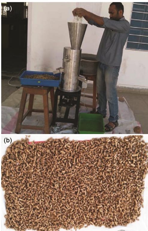
Fig. 7 — (A) Performance evaluation of developed feed pelleting machine; (B) 23 mm length and 10 mm Dia feed pellets produced
