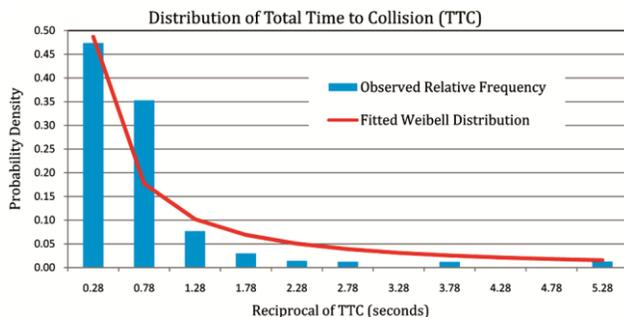
Fig. 3 — Distribution of Total Time to Collision (TTC) for midblock sections
