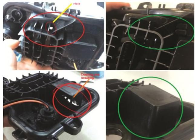
Fig. 2 — Sample defective product images which belong to injection process
