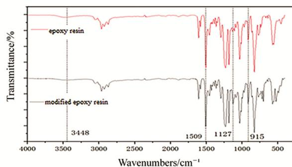
Fig. 4 — FTIR of silicone modified epoxy resin
