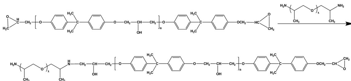
Fig. 2 — Curing reaction of epoxy resin
