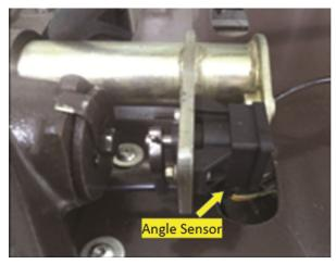
Fig. 5 — Placement of angle sensor
