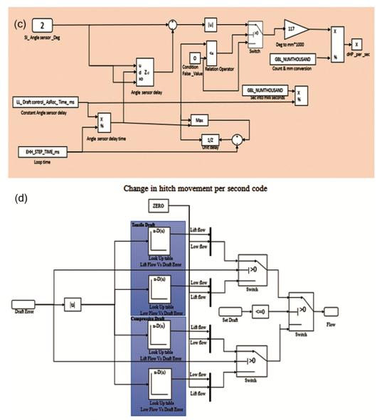
Simulink code to generate flow based on error draft
