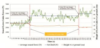
Fig. 11 — Performance and response time of the developed system
