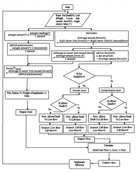
Fig. 6 — Control algorithm of EHH system through lower link draft sensing
