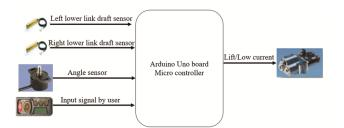
Fig. 1 — EHH systems through lower links draft sensing architecture
