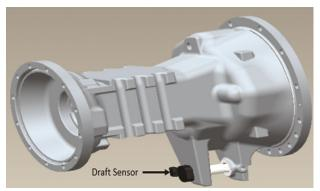
Fig. 4 — Isometric view for position of the draft sensor
