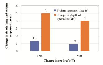
Fig. 13 — System response time with change in draft
