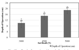
Fig. 12 — Depth of operation with set draft variation
