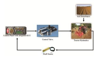
Fig. 2 — EHH system using lower links draft sensing as a closed loop system
