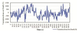
Fig. 10 - Variation of sensed force from set draft with time
