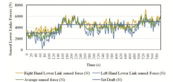
Fig. 9 — Variation of sensed lower link force with time
