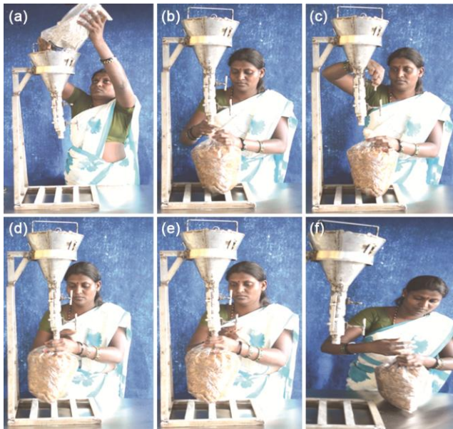
Fig. 4 — Sequence of manual operation of spawn spreading machine: (a) feeding of mushroom spawn inside hopper, (b) removing of cotton plug of the PP bag, (c) turn on and off the first valve for filling the spawn inside measuring jar, (d) inserting bag on the outlet end of machine, (e) turn on and off the second valve for inoculation and random spreading of the spawn on top of the substrate surface, (f) inserting cotton plug after inoculation
