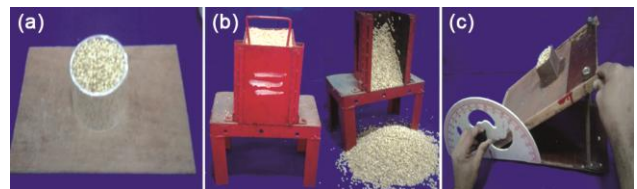
Fig. 1 — Determination of physical and engineering properties of mushroom spawn: (a) bulk density of spawn, (b) angle of repose of spawn, (c) coefficient of static friction of spawn
