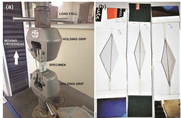
Fig. 4 — (a) Set up for tensile strength test (b) Single fibre specimen for tensile strength test
