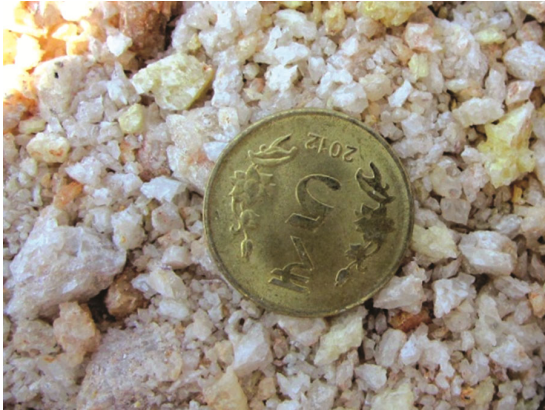
Fig. 6 — Typical medium hard rock for drop weight tests
