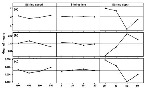
Fig. 3 — Mean main effect Plots for (a) Porosity, (b) Tensile strength, and (c) Loss of wear rate based on the parameters (i) Stirring speed (ii) Stirring time and (iii) stirring depth
