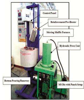
Fig. 2 — Vacuum-based squeezed stir casting setup
