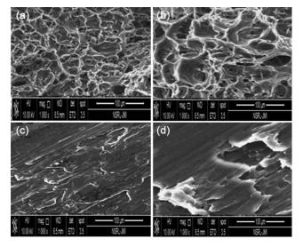
Fig. 12 — Microscopic image of tensile fracture (a & b) and Worn surfaces (c & d) of Mg-based  $S_{10}$  and  $S_{15}$  specimens
