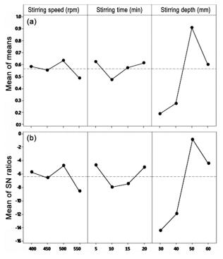
Fig. 6 — Mean main effect plots of (a) Composite desirable values (b) Signal to noise ratio of composite desirable values
