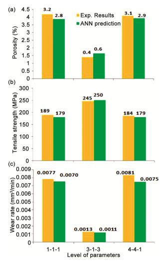
Fig. 11 — Compared results of experimenting and networking model of (a) Porosity, (b) Tensile strength and (c) Loss of wear rate
