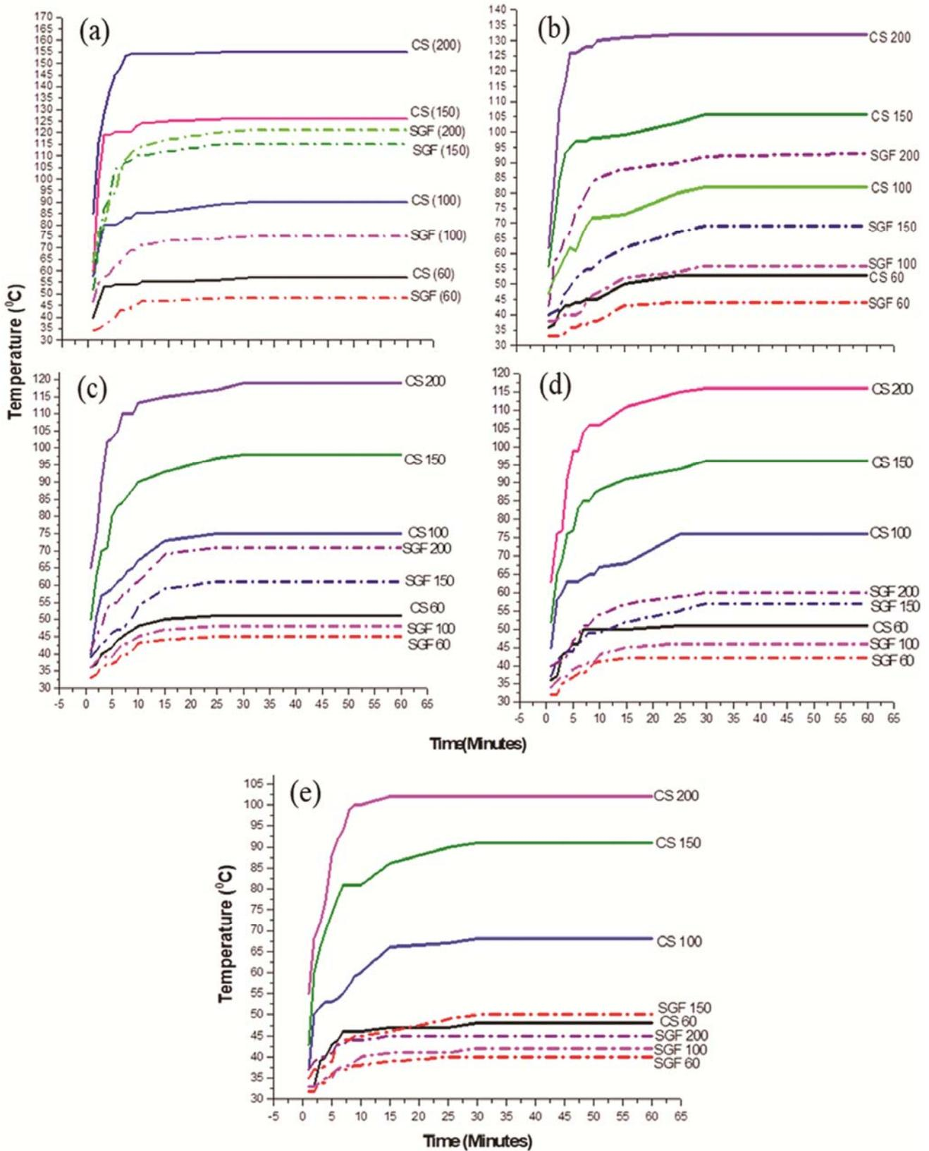
Fig. 1 — Comparative data of CS Vs SGF sheets of varying thickness 2 (a), 4 (b), 6 (c), 8 (d) and 10 (e) mm
