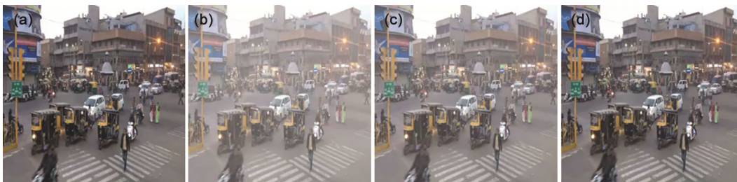
Fig. 12 — Video dehazing results for (a) input video, (b) hazy video with \beta = 0.6 , (c) result of existing method, average PSNR: 22.5, (d) result of proposed method, Average PSNR: 26.8
